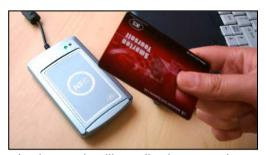
The ACR122S is the serial interface (RS-232) extension of the ACR122 Series, which is a family of NFC contactless smart card readers/writers. Developed based on the 13.56 MHz RFID technology and the ISO/IEC 18092 NFC standard, it also supports FeliCa and NFC tags, aside from MIFARE® and ISO 14443 Type A and B cards.
